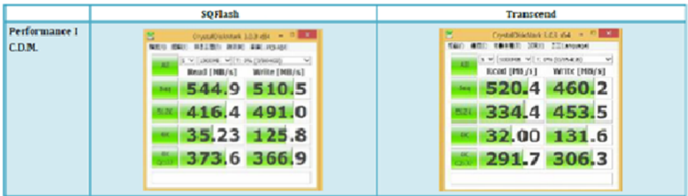
Fig 1. Performance I: Crystal Disk Mark performance comparison between SQFlash 830 vs Transcend 370 model
